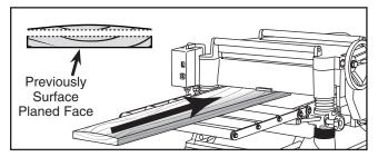
**3. Edge Joint On The Jointer**—The concave edge of the workpiece is jointed flat with the jointer.
